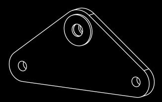
When using multiple sling legs this device provides a means of equalising forces within the legs. Connection is made via standard Grade "S" bow shackle and can be used with chain, wire rope or synthetic slings. Ideal in compensating for differences in load lift points and sling lengths.
